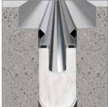
NEXUS Fire Barriers for horizontal expansion joint gaps with minimum movement capacity 50% of the joint width. Designed for Floor to Floor Gaps for 2 hours fire rated requirement and suitable for gap widths ranging from 35 - 350mm.
