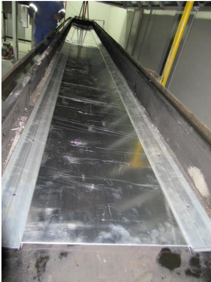
Photo 1: Specimen before the test. (Non-Fire Side)
